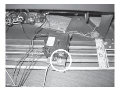
12) Install the supplied battery into the DC Sparker Box by opening the battery compartment.
